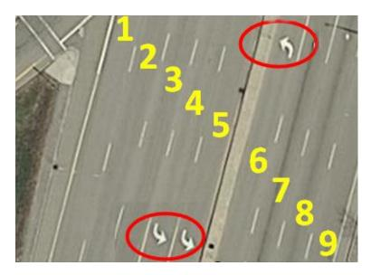
In this example, this roadway would be documented as a four lane roadway with one auxiliary lane. Notice the continuous-shared-left-turn lane is only counted as one lane.
