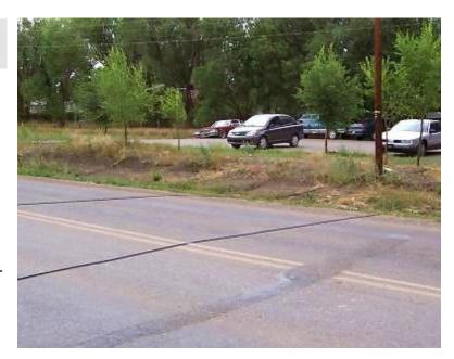
Constructed of several pressurized rubber hoses and a specialized counting device, a traffic counter can count either the number of axles or the number of vehicles that cross-over the counter.
