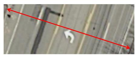
Roadway width, measured from edge of pavement to edge of pavement, including the maintained and surfaced shoulders on each side. Notice the shared-left-turn lane  ${\bf is}$  included in the roadway width.
