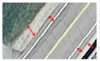
In this case SHLDR\_RIGHT would be recorded as '4' and SHLDR\_LEFT would be recorded as '6'.
