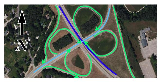
Interchange between NH 16 (shown in dark blue) and NH 9 (**shown in light blue**) in Dover. Each ramp (**shown in green**) is not a slip ramp. Despite single directions of access and egress, none of the ramps divide, and are therefore classified as primary ramps
